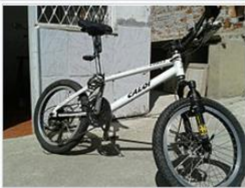
An aluminum BXR bike made by Caloi and built using Shimano Acera and 27 Speed and a wheelset with 36 spoke count.
